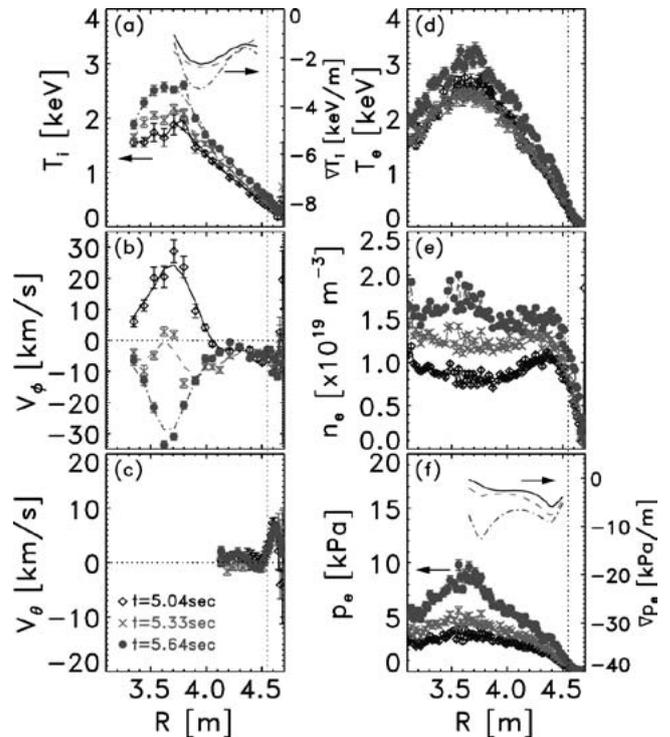
Fig. 2. Profiles for (a) ion temperature, (b) toroidal, (c) poloidal rotation for carbon impurity ions, electron (d) temperature, (e) density, and (f) pressure vs. major radius.
