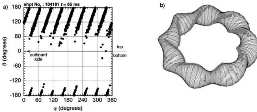
**Figure 3.** (a) Spatial distribution of beam ion losses in Cartesian coordinates. (b) 3D plot of beam ion losses on the last closed flux surface of CHS in  $B_t/R_{\text{ax}} = 1.9 \text{ T}/0.921\text{m}$ .
