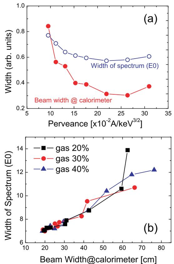
Fig. 5 (a) The beam width measured by the calorimeter and the line width of full energy beam component. (b) The correlation of them in the cases with the gas fueling rate of 20%, 30% and 40%.
