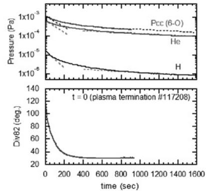
Fig. 2. Time evolution for pressures and divertor temperature in the vacuum vessel just after high-performance long-pulse discharge.
