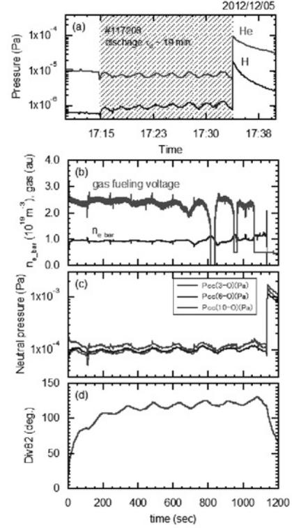
Fig. 1. Hydrogen and helium pressure, gas fueling, line averaged electron density, neutral pressure ( $P_{cc}$ ) and divertor temperature during the long-pulse discharge.
