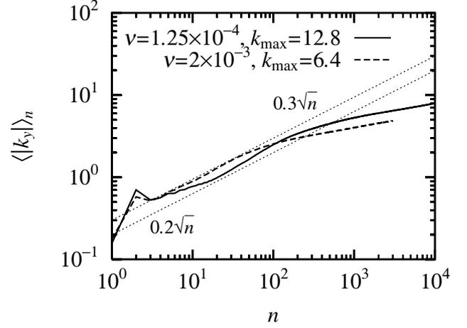
Fig. 1 Spectrum-averaged wave number  $\langle |k_y| \rangle_n$  for  $(k_{\text{max}}, \nu) = (6.4, 2 \times 10^{-3})$  and  $(k_{\text{max}}, \nu) = (12.8, 1.25 \times 10^{-4})$ . Upper and lower dotted straight lines represent  $\langle |k_y| \rangle_n = 0.3\sqrt{n}$  and  $0.2\sqrt{n}$ , respectively.
