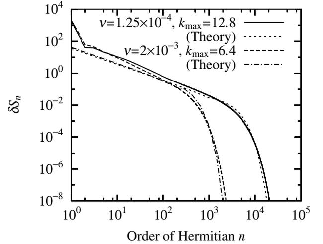
Fig. 2 Entropy spectra  $\delta S_n$  (solid and dashed lines) obtained by the same simulation as in Fig. 1. For comparison, dotted and dot-dashed lines represent the combination of eqs. (10) and (11). Here, eq. (10) is used for  $n < 3 \times 10^2$  ( $10^3$ ) and eq. (11) for  $n > 3 \times 10^2$  ( $10^3$ ) in the case of  $k_{\text{max}} = 6.4$  (12.8).
