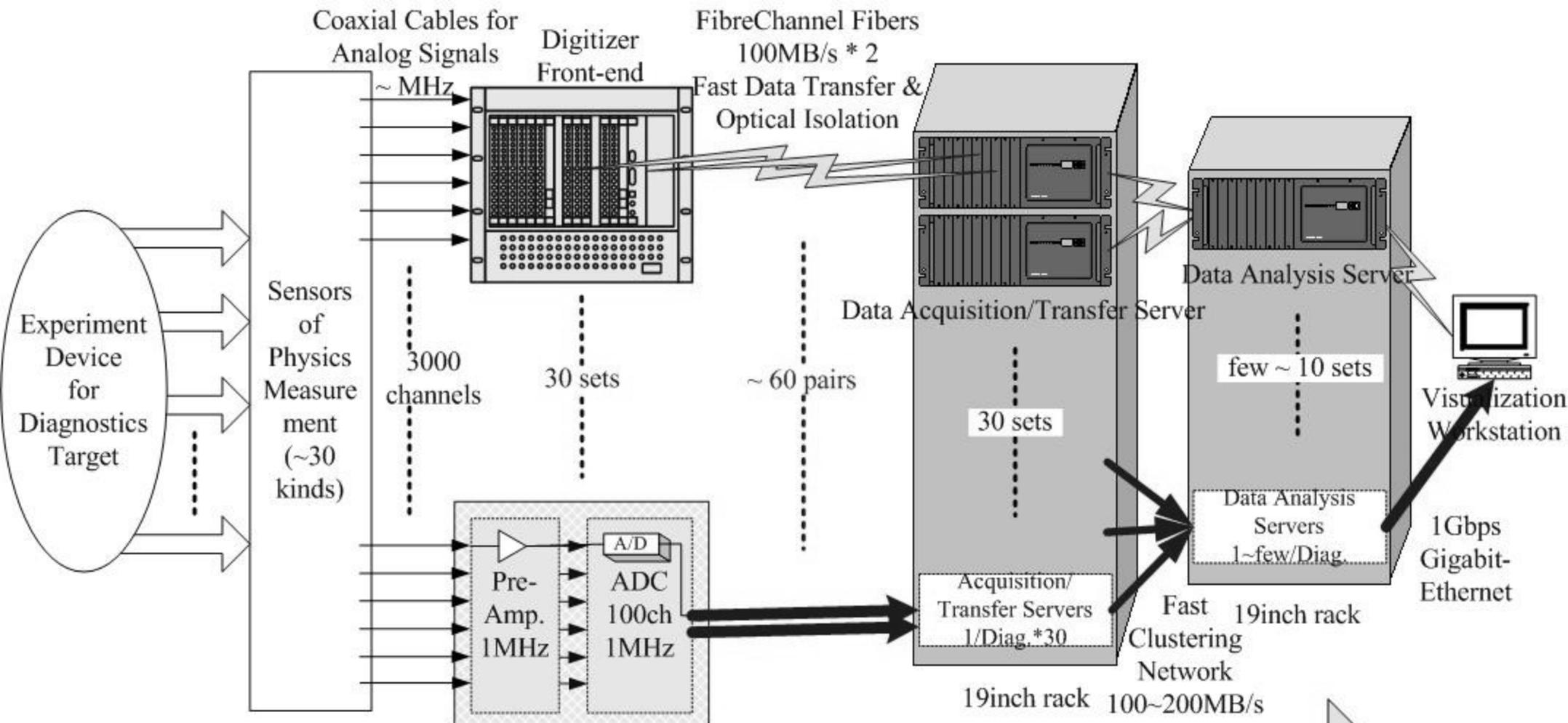
*Ultra-Fast (100~200MB/s) (1MHz/ch) Non-Stop Data Transfer = Real-Time Data Streaming*
