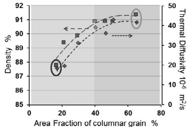
Fig. 1: The dependence of the density and thermal diffusivity of the VPS-W on the areal fraction (%) of columnar grains in the cross sectional area of VPS-W
