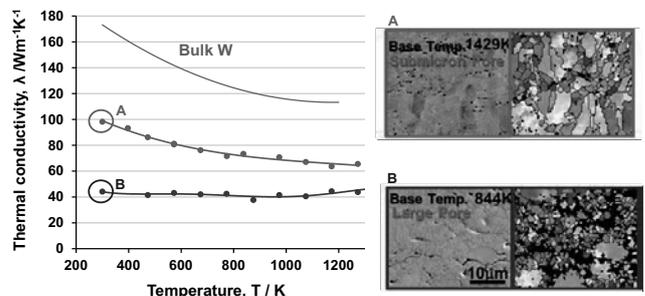
Fig. 2 : Correlation of thermal diffusivity with grain morphology of VPS-W
