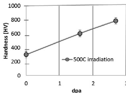
Fig. 2: Dose dependence of irradiation hardening of VPS-W irradiated at 773K.
