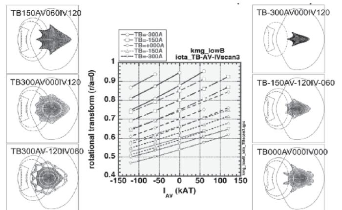
Fig. 2. Feasible magnetic configurations and the relation between coil currents, rotational transform and magnetic flux surfaces in a low magnetic field operation
