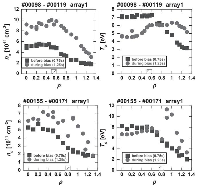
Fig. 1. Radial profiles (before/after biasing) of electron temperature  $T_e$  and electron density  $n_e$  measured by the triple probe. The electrode positions were  $r = 0.5$  and  $0.75$ .
