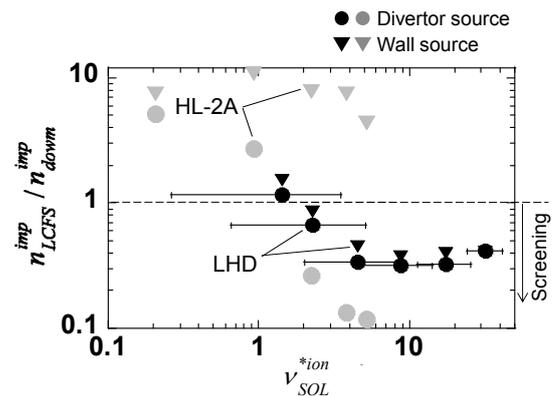
Fig. 1. The ratio  $n_{LCFS}^{imp}/n_{down}^{imp}$  as a function of collisionality. Circles: impurity released at the divertor plate, triangles: impurity released at the first wall, for LHD (black symbols) and HL-2A (grey symbols).
