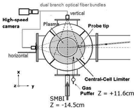
Fig.1. Schematic view of the central-cell cross-section and the locations of SMBI system and high-speed camera
