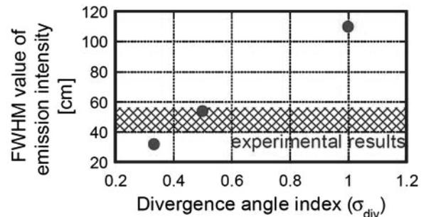
Fig.4. Comparison of FWHM value of emission intensity between experimental results and simulation results.
