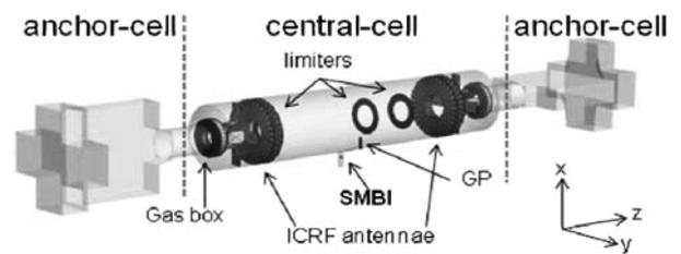
Fig.3. A fully 3-dimensional DEGAS mesh model with SMBI port.
