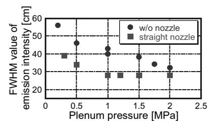
Fig. 2. FWHM of emission intensity from camera image as a function of plenum pressure.
