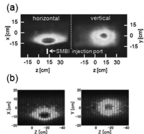
Fig. 1. (a) Fast camera image of the visible emission during SMBI and (b) 2-D  $H\alpha$  image calculated by simulation.
