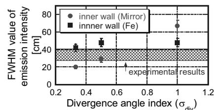
Fig. 3. FWHM of emission intensity by simulation as a function of divergence angle index.
