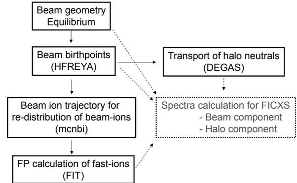
Fig. 1. Calculation scheme for the estimation of the fast ion charge exchange spectrum.
