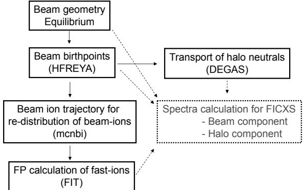
Fig. 1. Calculation scheme for the estimation of the fast ion charge exchange spectrum.
