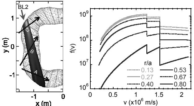
Fig. 2. (Left) 2-dimensional beam density of co (BL2) NBI and sightlines of the test geometry for the FICXS spectrum calculation and (Right) velocity distribution of fast ions at  $r/a = 0.1$  to 0.8 calculated by the Fokker-Planck analysis.
