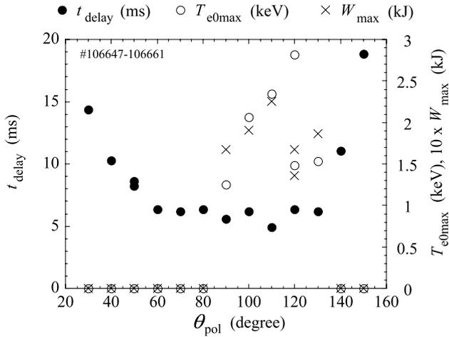
Fig. 3 The time delay of density start up  $t_{delay}$  (closed circle), the maximum stored energy  $W_{max}$  (cross) and the highest central electron temperature  $T_{e0max}$  (open circle) achieved during the plasma duration are plotted as functions of the polarization direction  $\theta_{pol}$ . Here,  $W_{max}$  is multiplied by 10 for convenience.
