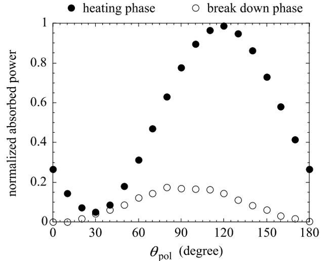
Fig. 4 Calculations of total absorbed power with various directions of linear polarization  $\theta_{pol}$  are plotted taking the injection power as unity. For the calculation of the break down phase, localized profiles of temperature and density around the magnetic axis, and for the heating phase nearly flat density profile and peaked temperature profile are adopted, respectively.
