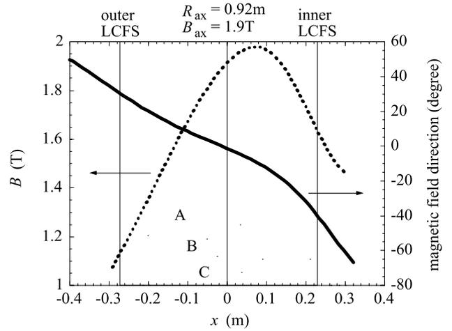
Fig. 2 The strength of magnetic field and the angle between magnetic field direction and toroidal direction along the beam path are plotted. The beam comes from negative  $x$  side. The curves marked as A, B show schematic profiles of  $n_e$  and  $T_e$  respectively used in latter calculations for heating phase, and C,  $n_e$  and  $T_e$  for break down phase.
