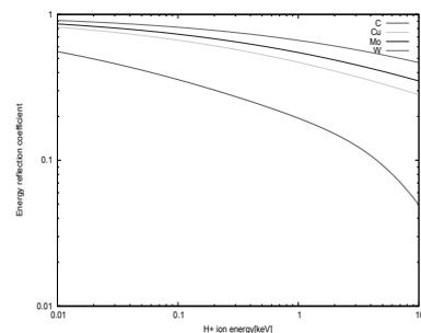
Fig. 3: Ion energy reflection coefficient evaluated with Eckstein's empirical formula.
