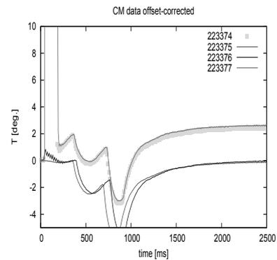
Fig. 2: Fast TC signal noise around GAMMA 10 plasma discharge. Normal discharge (#223374, #223377), only seed plasma without RF heating (#223376), and only magnetic field (#223375).
