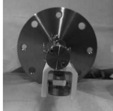
Fig. 1: Constructed calorimeter head.
