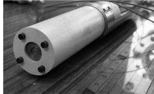
Fig. 2: Photo of combined probe with a Cu GTP tip.
