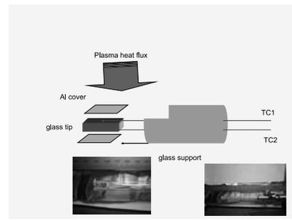
Fig. 2: Basic design of glass GTP tip. Both area is covered with thin Ar film and connected with the junction point of Type-K thermocouple.
