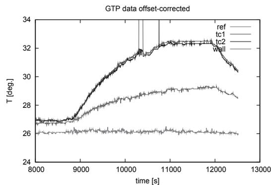
Fig. 3: Raw data of GTP thermocouple (front: red solid line, back: blue dotted line). The offset of these signals are corrected. Reference signals for room temperature and chamber wall temperature are also plotted.
