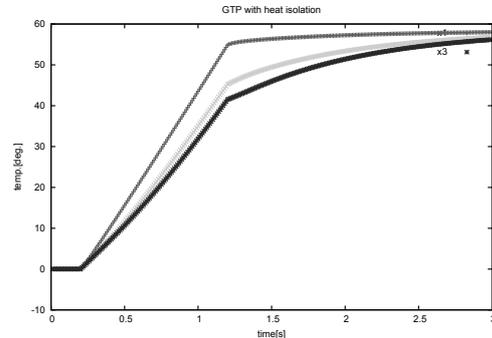
Fig. 1: Calculation of temperature response of a Cu GTP tip without the heat sink.
