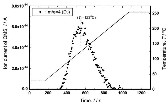
Fig. 2 An example of desorption spectra of deuterium.
