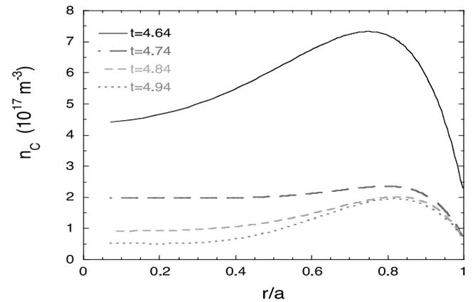
Fig.1 Measured carbon density profile at four times following TESPEL injection in shot 113208.
