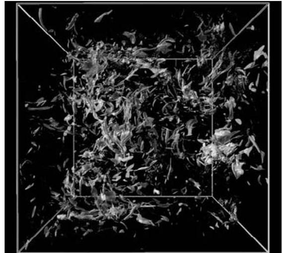
Fig. 1: The enstrophy density (square of the vorticity vector) and the Laplacian of the magnetic pressure are drawn in the colored and grey isosurfaces, respectively.
