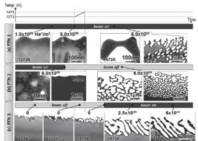
Fig. 2. The microstructural evolution of the edge parts of W under the three different irradiation conditions
