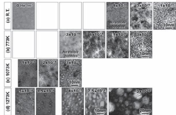
Fig. 1. The microstructural evolution of W under the 3 keV-He<sup>+</sup> irradiation at constant temperatures
