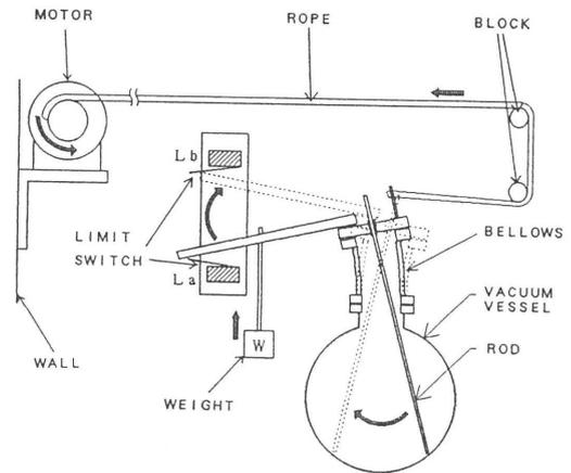
Fig. 1. Rod scanning R&D system for magnetic surface mapping in LHD.
