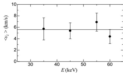
Fig. 3 The  $\langle v_z \rangle$  value of  $\text{W}^*(6p^7\text{P}_4)$  atoms as a function of projectile energy.
