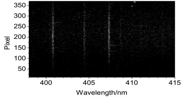
Fig. 1 A typical IBLE spectrum of a polycrystalline tungsten surface bombarded by  $\text{Kr}^+$  ion beam.
