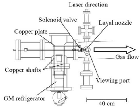
Fig. 1. Schematic of the experimental setup. A solenoid valve installed in the vacuum chamber is cooled by the GM refrigerator through copper plates.
