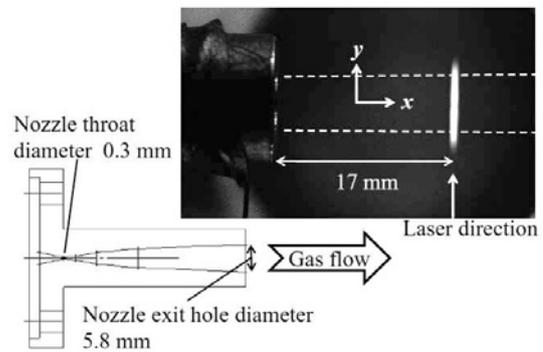
Fig. 2. Typical CCD image in the case of  $\text{H}_2$  at 125 K and the cross section of the Laval nozzle. The backing pressure is 8.0 MPa, and the exposure time is 10 ms. The laser beam direction ( $y$ ) is perpendicular to the gas flow ( $x$ ). The broken lines denote extension of the exit hole with a diameter of Laval nozzle (5.8 mm).
