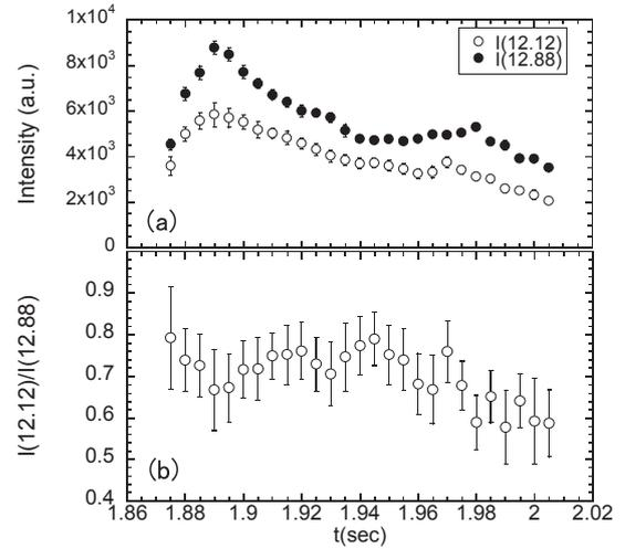
Fig. 2. Temporal distribution of (a) the line intensities of  $I(\lambda 12.12\text{nm})$  and  $I(\lambda 12.88\text{nm})$  and (b) the line intensity ratio.
