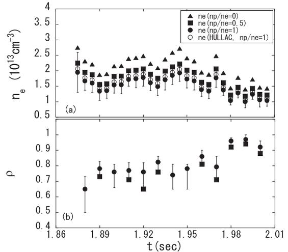
Fig. 3. Temporal distribution of (a) electron density estimated from the measured intensity ratio and CR model, and (b) normalized radius  $\rho$  of location of emitting region for different models (RMaX model with  $T_e=1.04\text{keV}$  and  $n_p/n_e=0$  (solid triangles),  $0.5$  (solid squares), and  $1$  (solid circles), and HULLAC model with  $T_e=1.04\text{keV}$  and  $n_p/n_e=1$  (open circles)). Errors are shown only for the RMaX model with  $n_p/n_e=1$ .
