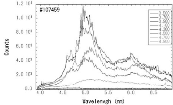
Fig. 1 EUV spectra measured in LHD plasmas. TESPEL was injected at  $t=3.8\text{s}$ . Central electron temperature changed from  $2.5\text{keV}$  ( $t=3.9\text{s}$ ) to  $0.3\text{keV}$  ( $t=4.5\text{s}$ ).
