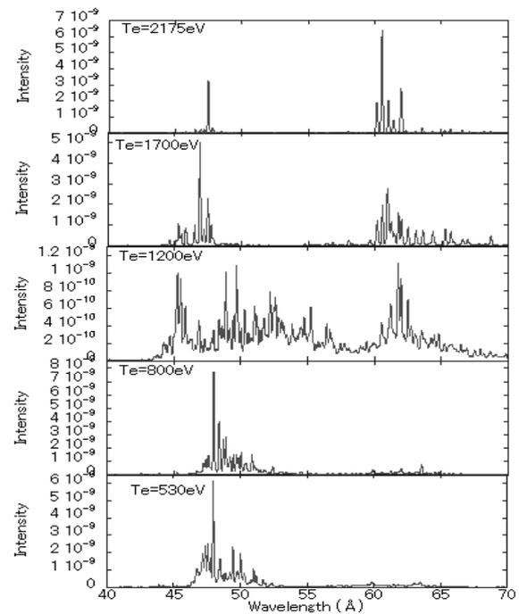
Fig. 2. EUV spectra calculated with CR models for electron temperature  $530\text{eV}$ ,  $800\text{eV}$ ,  $1200\text{eV}$ ,  $1700\text{eV}$  and  $2175\text{eV}$  from bottom to upper panels with electron density  $10^{13}\text{cm}^{-3}$ . Ionization equilibrium is assumed for ion abundances.
