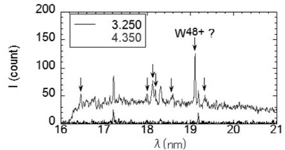
Fig. 3 EUV spectrum at wavelength region  $\sim 16 - 21\text{nm}$  taken by SOXMOS for #112877 at  $t=4.35\text{s}$ . Several tungsten lines are found.
