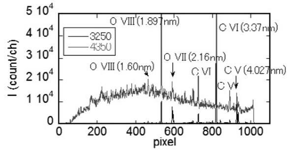
Fig.1 EUV spectrum at wavelength region  $\sim 0 - 4.5\text{nm}$  taken by an EUV spectrometer for #112877 at  $t=4.35\text{s}$  and  $t=3.25\text{s}$  before a TESPEL injection. Continuum is increased maybe due to radiation from tungsten ions.
