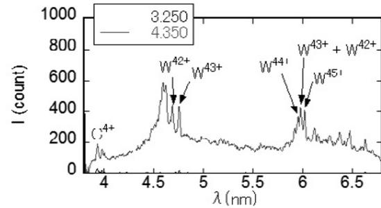
Fig.2 EUV spectrum at wavelength region  $\sim 4 - 6.8\text{nm}$  taken by SOXMOS for #112877 at  $t=4.35\text{s}$ . Discrete lines of  $W^{42+} \sim W^{45+}$  ions are identified.
