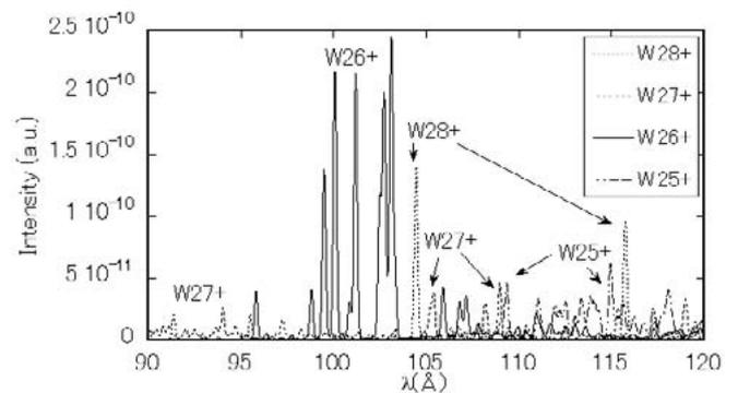
Fig. 3 Calculated EUV spectra for the same wavelength region as Fig.2 for W<sup>25+</sup> to W<sup>28+</sup> ions using the collisional-radiative models with assumption of electron temperature 700eV and electron density 5x10<sup>13</sup>cm<sup>-3</sup>. Isolated lines are produced for W<sup>26+</sup> ion, which correspond to the peaks seen Fig. 2 at around 10nm.
