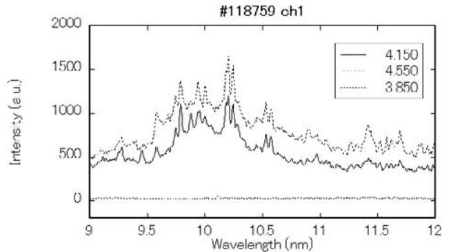
Fig.2 EUV spectrum at wavelength region of 9 - 12 nm taken by SOXMOS for #118759 at t = 4.15 and 4.55 s. Several isolated peaks are observed at around 10nm, which are predicted by CoBIT measurement.
