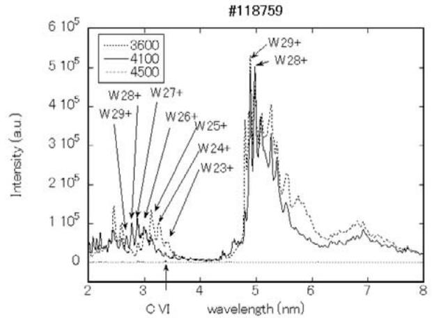
Fig.1 EUV spectrum at wavelength region of 2 - 8 nm taken by an EUV spectrometer for #118759 after a TESPEL injection. Spectral peaks of n = 5 - 4 transitions from W<sup>23+</sup> - W<sup>29+</sup> ions are identified.
