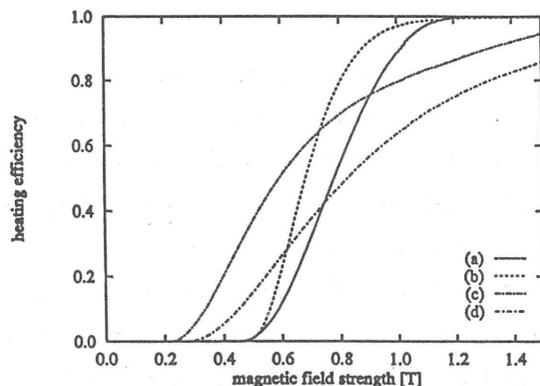
Fig. 1: Heating efficiencies of tangentially injected NBI heating in the CHS as a function of the magnetic field strength,  $B$ , for configurations with different  $\beta$ ; (a)  $\beta = 0.0\%$ , (b)  $\beta = 0.84\%$ , (c)  $\beta = 1.83\%$ , and (d)  $\beta = 2.38\%$ .
