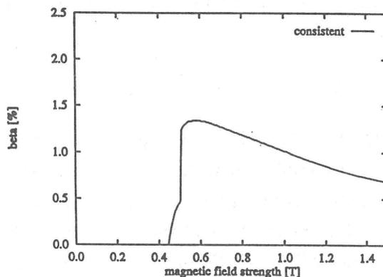
Fig. 2: Plots of the averaged beta values,  $\beta$ , as a function of the magnetic field strength,  $B$ , using the consistent configurations with obtained  $\beta$  values.
