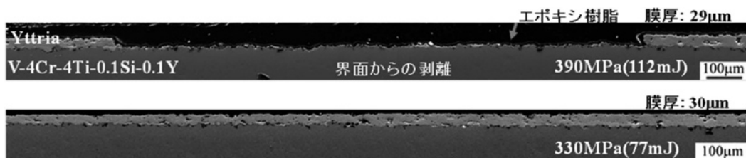
Fig. 2 Scanning electron microscopy of the cross-section of interface between yttria and vanadium alloys.
