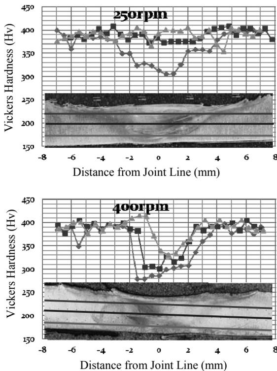
Fig. 1 Cross-sectional Vickers hardness distributions in F82H/ODS joints joined by FSW.
