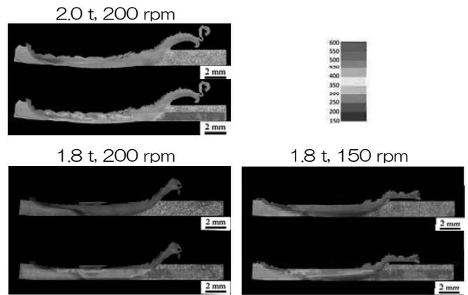
Fig. 2 Cross sectional Vickers hardness distributions in F82H/12Cr-ODS joints joined by FSW.
