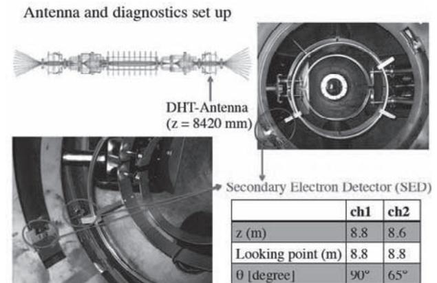
Fig. 1 DHT antenna and SED in the edge region of the GAMMA 10 device.
