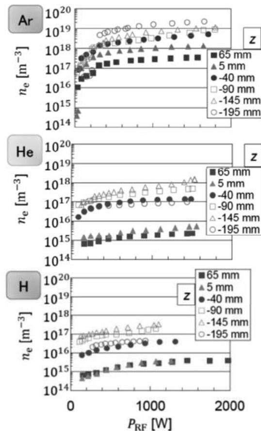
Fig. 1. Dependence of electron density on RF power, changing gas species.
