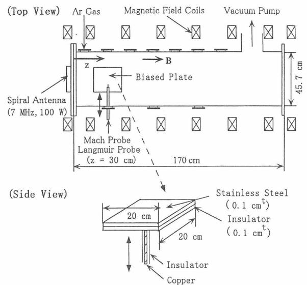
Fig. 1. Schematic view of experimental setup
