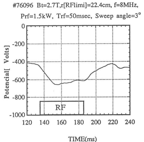
Fig. 2 Time variation of plasma potential at 2°. Prf=1.5 kW, f=8 MHz.
