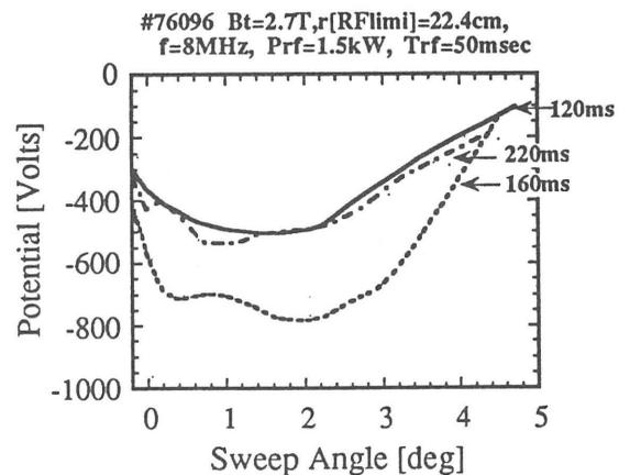
Fig. 3 Spacial profiles of plasma potential before, after the RF and during the RF.
