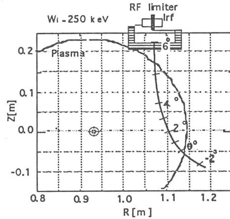
Fig.1 Coordinate of potential measurement for 250 keV TI beam and the RF limiter position.
