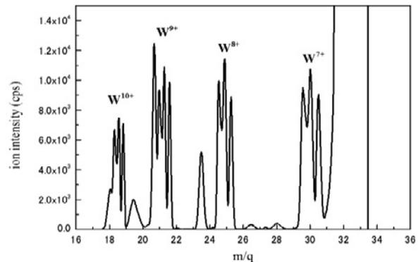
Fig. 2. Mass spectrum in introducing  $W(CO)_6$ .
