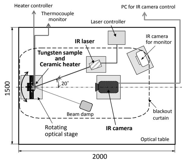
Fig. 1 Experimental setup: Tungsten sample mounted on the rotating optical stage is heated by a ceramic header put on the back of the sample. The sample is irradiated by an IR laser and the scattered light on the surface is measured by an IR camera.
