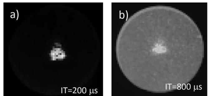
Fig.2 Images of IR camera for tungsten samples with a) a sandblasted surface and b) a mirror surface. Surface temperatures and the integrated times are 277°C and 200  $\mu\text{s}$  for a), and 272°C and 800  $\mu\text{s}$  for b) respectively.
