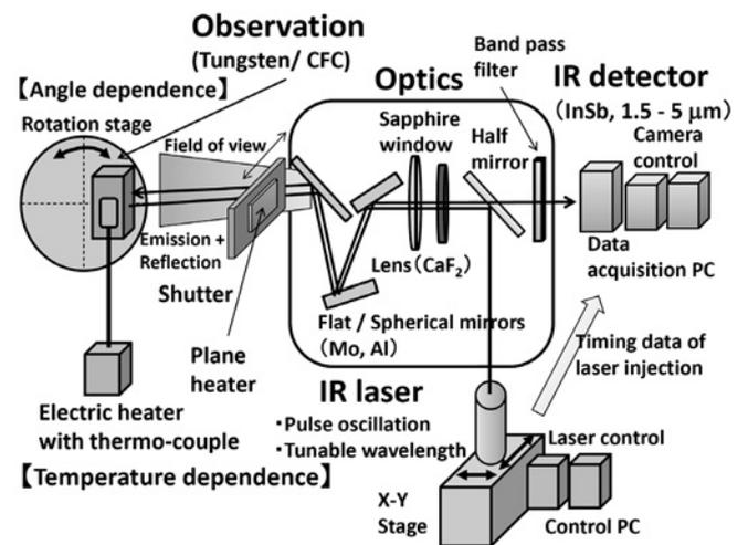
Fig. 1 Conceptual diagram of proof-of-principle experiment for in-situ calibration technique of infrared camera measurement
