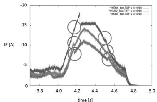
Fig. 2: Results of the biasing experiment with different perturbed field. Increasing the island width, the current to transit is also increased.
