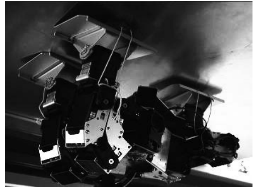
Fig. 1: The inverted walking on the roof by using the suckers.
