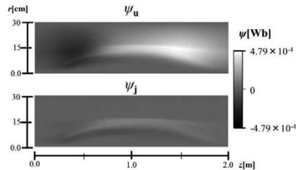
Fig. 2. 2D profile of increment of magnetic flux. Due to (Top) the Lorentz force and (Bottom) the resistive force
