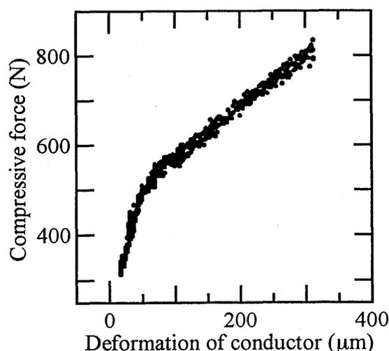
Fig. 2: Deformation of conductor due to transversal compressive force.
