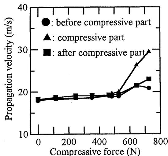
Fig. 3: Propagation velocity of normal zone.
