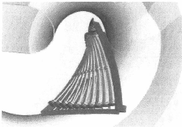
Fig. 1. A drawing of the stacked comblines antenna inside the LHD vacuum vessel. The grounded ends of the top and bottom comblines are located on the midplane. The Faraday shield elements and the side protection tiles are removed for ease of viewing.
