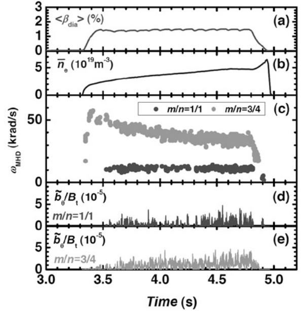
Fig. 1. MHD activities in the discharge with  $\langle\beta_{\text{dia}}\rangle \sim 1.5\%$ . (a) the volume averaged beta value, (b) line averaged electron density, (c) angular frequencies of MHD modes, amplitudes of (d)  $m/n = 1/1$  and (e)  $3/4$  modes.
