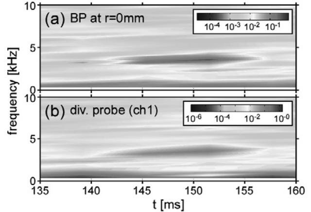
Fig. 2. Spectrograms of (a) beam current at the center and  $I_{\text{sat}}$  at ch. 1.
