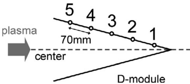
Fig. 1. Schematic diagram of divertor module with Langmuir probes.
