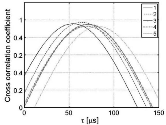
Fig. 3. Cross correlation coefficients between band-passed fluctuations of beam current and  $I_{\text{sat}}$  at ch. 1–5 (blue, green, red, cyan, and magenta).
