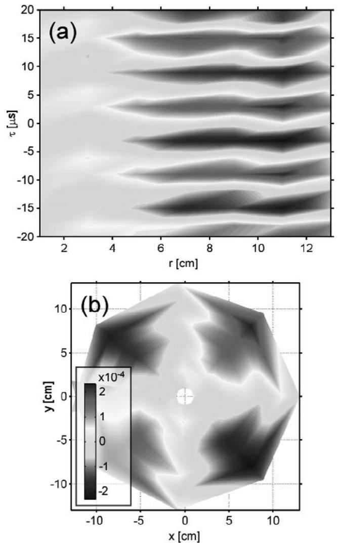
Fig. 1. (a) Cross-correlation function of floating potential at the target plate and band-passed plasma potential measured with GNBP as functions of  $r$  and  $\tau$ . (b) Converted image of the cross-correlation by using Eq. (1).
