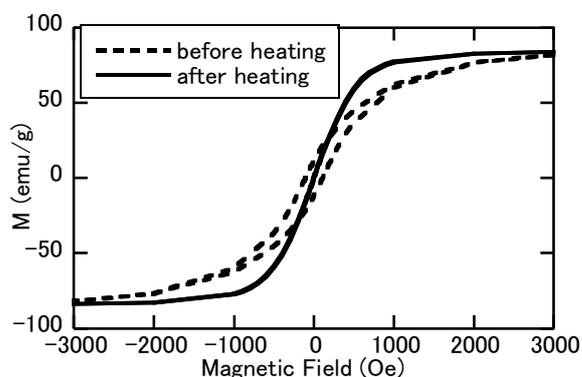
Fig. 3. The hysteresis loop of the magnetite sintered by using magnetic field of microwave at 1000 °C.
