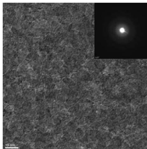
Fig. 2. A transmission electron microscope image of a sintered body of magnetite powders by the microwave magnetic field heating.
