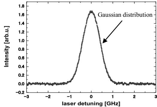
Fig.2. LIF spectrum for argon neutral particles.
