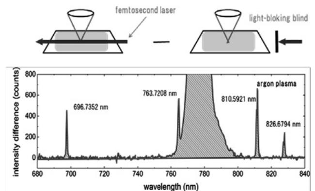
Fig.2 Spectrum increment caused by femtosecond laser pulses. Scattered light from the femtosecond laser is overwritten (760-800 nm)
